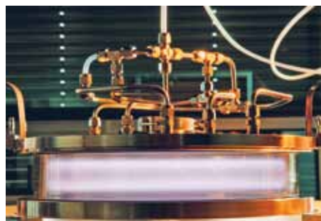
Environmentally friendly plasma technology is an alternative to conventional wet chemical textile processing. (Source: Empa)
