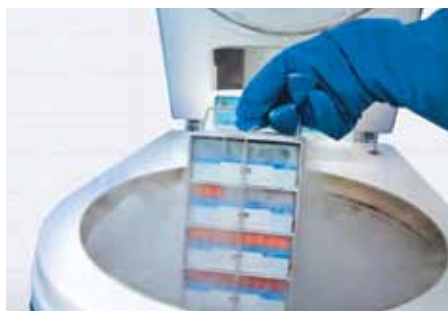
In the Culture Collection of Switzerland (CCOS) bacterial strains are stored in liquid nitrogen at -196\text{ }^{\circ}\text{C} . (Source: CCOS)
