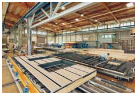
Production of a prefabricated wooden element. (Source: Renggli AG)
